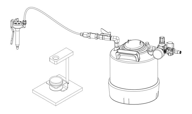
System shown above includes optional PV105-1 Valve Stand with solvent/purge cup.
