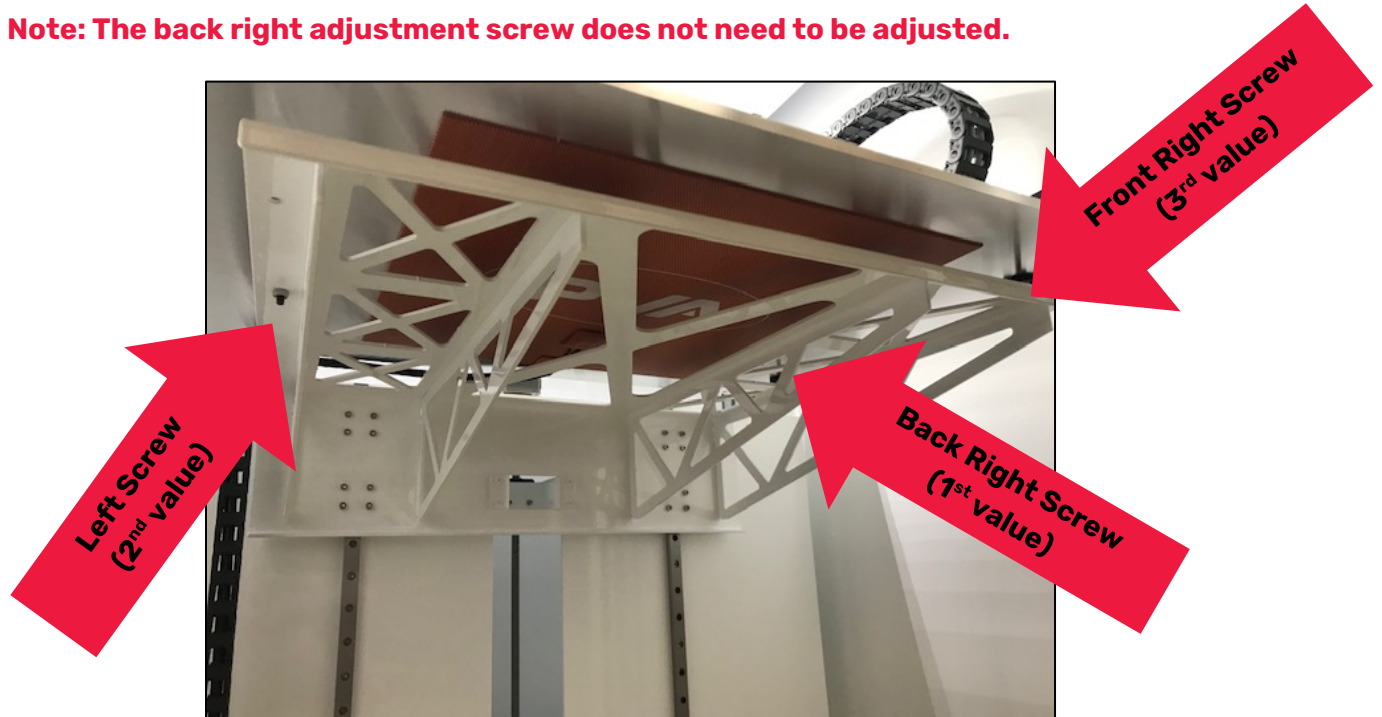
Figure 18: Three Leveling Screws
