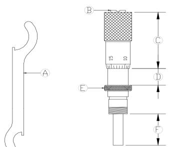
Figure 3: Micrometer Adjustment Breakdown
