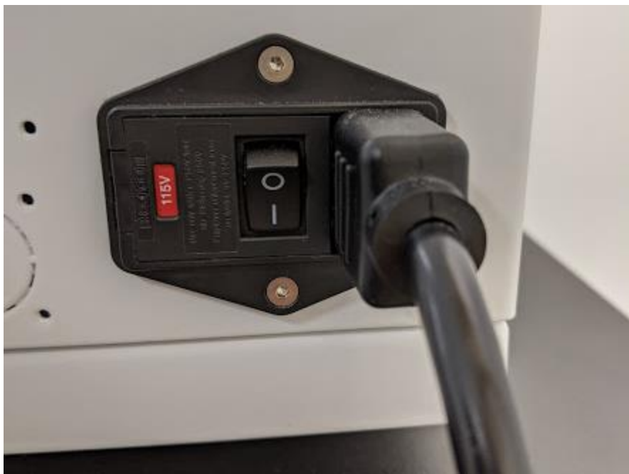
Figure 3: Main Power Switch
